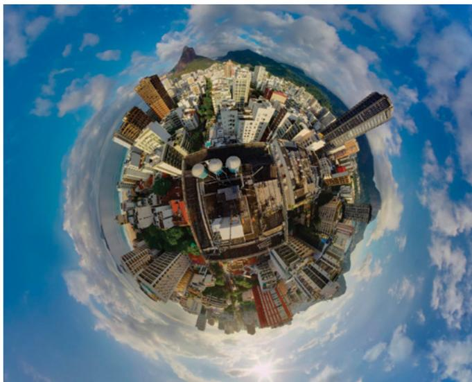
Figure 1. Full Sphere Panoramic Image in a Stereographic Projection
